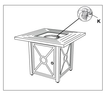
Before performing a leak test, be sure that no sparks can occur and you are in a spacious outdoor area. Connect the propane gas tank to the regulator and turn the valve on the unit to the "off" position. Brush a soap and water mixture on all connections. Turn the gas supply on; if bubbles occur on any connection there may be a leak. If you smell gas or a leak is discovered turn the gas valve off, disconnect propane gas tank and do not use the appliance until the leak is repaired.
